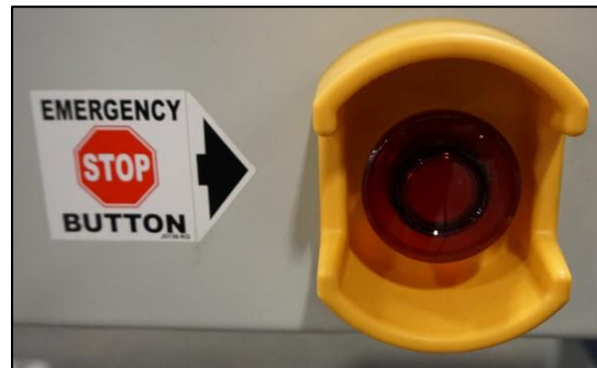
Figure 1 – Emergency Stop (E-Stop) Button
